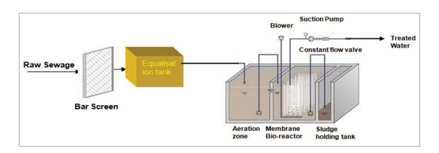
Figure 3: Treatment of Sewage Using Membrane Bio-reactor
