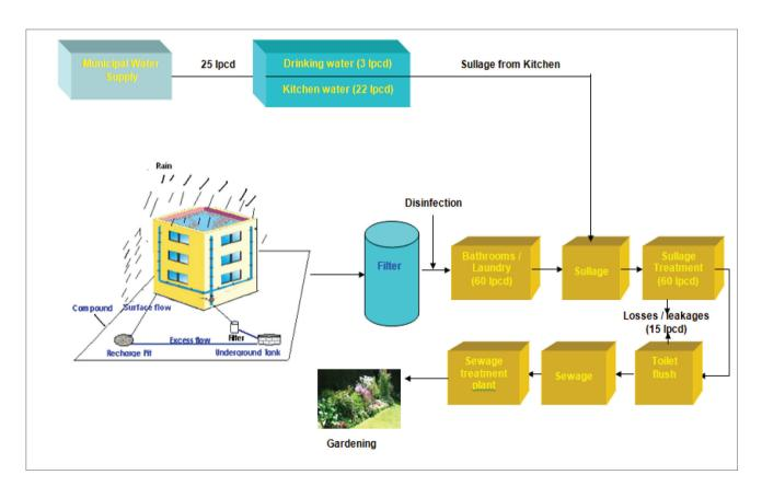
Figure 1: Total Water Management In Residential Complexes Using Rain Water And Sullage
