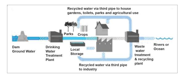
Figure 5: Water Recycling For Non-Drinking Uses
