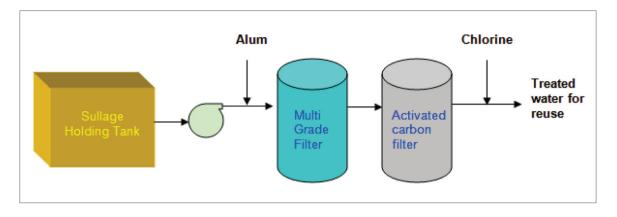
Figure 2: Sullage Recycle System
